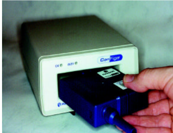
Figure 3 - A TransPondIT being configured in a ConFigIT
