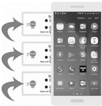
Open the Blutag app and place your device in contact with the data logger. You will be directed to the main page where you can access information about the data logger.
