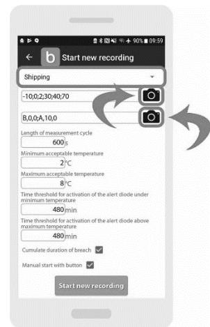
For all the profiles you can also choose length of measurement cycle, time thresholds for activating the alert diodes, temperature limits, cumulating duration of breach, PIN codes, manual start or delay of start.
