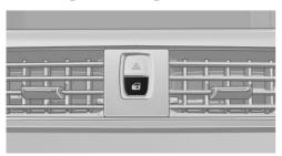
Pressing the central locking system button locks or unlocks the vehicle with the front doors closed.
