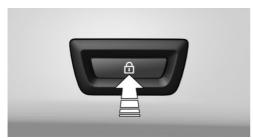
Press the button on the inside of the trunk lid to lock the vehicle prior to closing.
