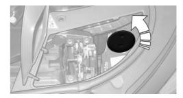
3. Unscrew the bulb holder counterclockwise.
