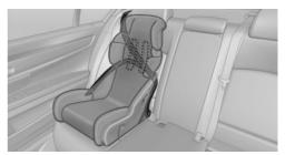
The rear safety belts and the front passenger safety belt can be permanently locked to fasten child restraint systems.
