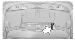
The tow fitting is located in the container on the inside of the trunk lid.
