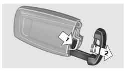
Press button, arrow 1, and remove the key, arrow 2.
