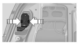
Squeeze the clips together and remove the bulb holder.
