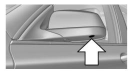
The lenses of the Top View camera are located at the bottom in the mirror housings. The image quality may be impaired by dirt.
