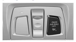
The indicator lamp for the front-seat passenger airbags indicates the operating state of the front-seat passenger airbags.
