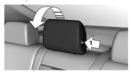
Press button, arrow 1, and fold the head restraint forward.
