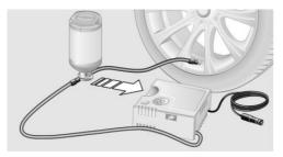
Screw the filling hose of the sealant container onto the tire valve of the defective wheel.
