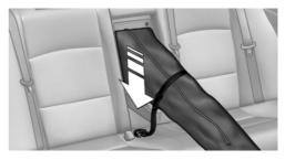
Tighten the retaining strap.
