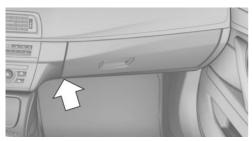
Socket is located below the glove compartment.
