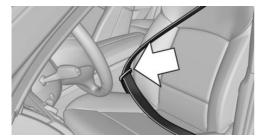
Make sure you hear the latch plate engage in the belt buckle.
