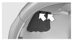
Remove the screws and fold down the lid.
