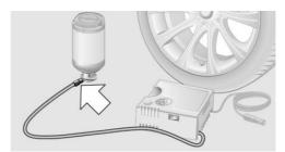
4. Insert the sealant container on the compressor housing in an upright position.
