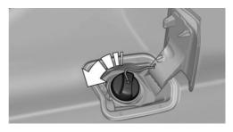
3. Place the tank lid in the bracket attached to the fuel filler flap.
