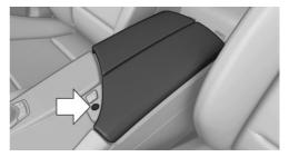
The storage compartment in the armrest can be locked with an integrated key to separately secure the trunk lid, refer to page 42, e.g.
