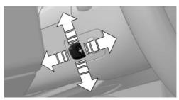
The steering wheel can be adjusted in four directions.
