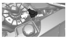
The so-called starting aid terminal in the engine compartment acts as the battery's positive terminal
