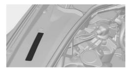
The vehicle identification number can be found in the engine compartment.
