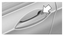
Touch the surface on the handle of a vehicle door, arrow, with your finger for approx. 1 second without grasping the door handle.
