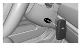
M double-clutch transmission: if a corresponding Check Control message appears, hold the remote control, as shown, against the marked area on the steering column and press the Start/Stop button within 10 seconds while pressing the brake.
