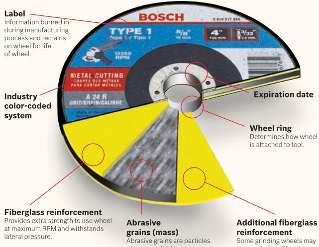
Abrasive grains are particles of man-made abrasive compounds. Bosch uses only high-quality grains.
