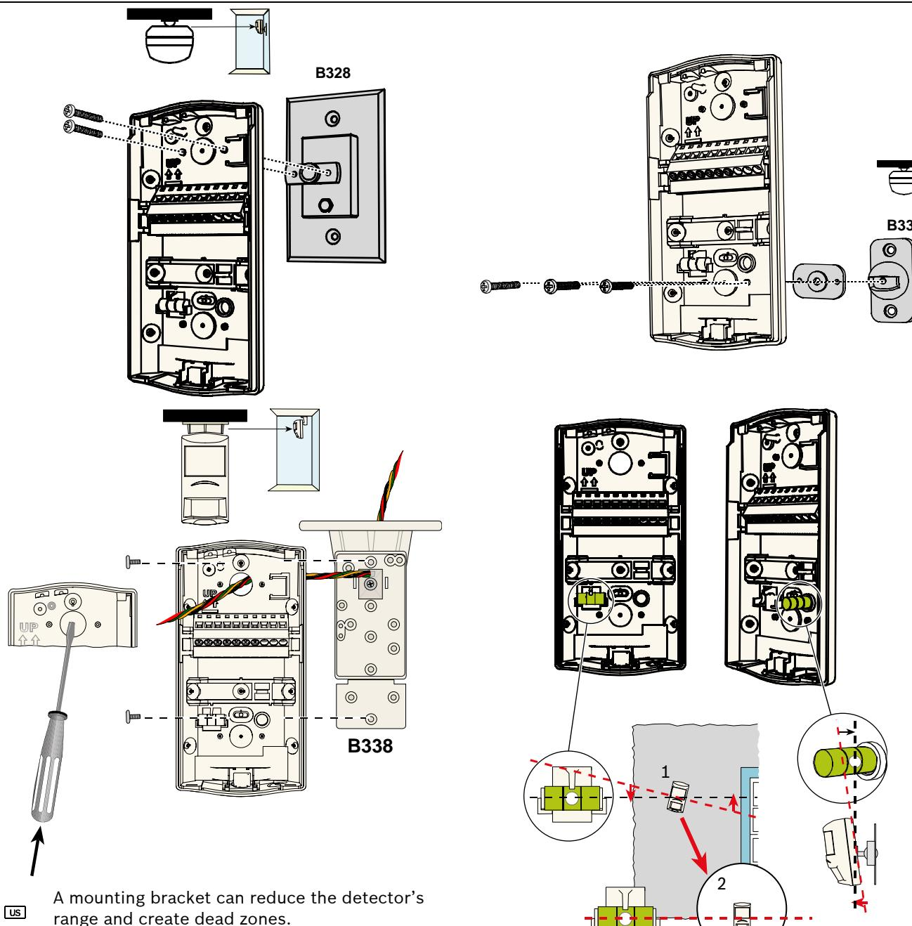
**[US]** A mounting bracket can reduce the detector's range and create dead zones.
