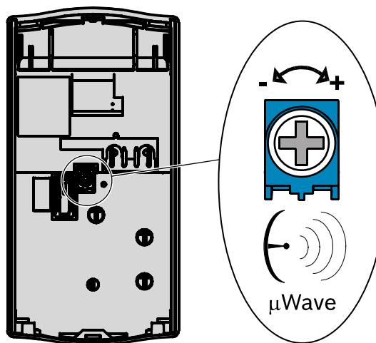
If necessary, adjust microwave range slightly until required coverage is met.
