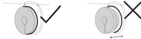
6. Place the camera base onto the surface mounting plate.
