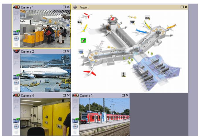
Displays a variable number of Image panes. Minimum is 1 Image pane. You can display one camera in several Image panes simultaneously.
