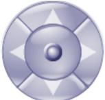
Click an arrow or drag the joystick in the center to swivel the camera in all directions.
