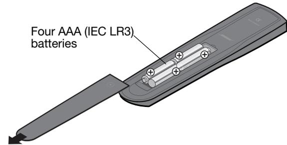
2. Install the four supplied batteries, matching the polarity markings (+ and -) on the batteries to the markings inside the battery compartment.
