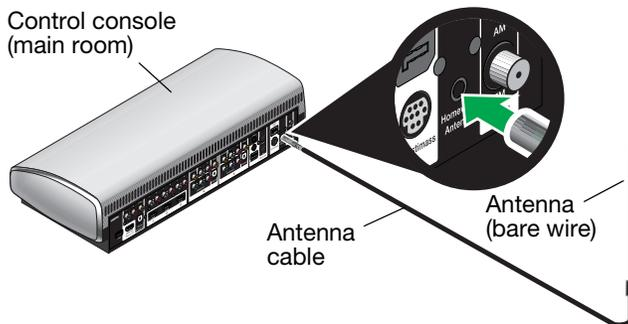
Because the antenna radiates at 90 degrees to the antenna (bare wire), mount the antenna vertically as close as possible to the center of the house.
