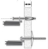
To mark mounting hole locations, remove the rubber feet, hold the amplifier in position, and mark the wall through the clearance holes in the housing.
