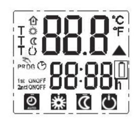
To start the controller fit two "AA" batteries in the battery compartment. Once batteries are fitted all symbols will be displayed on the LCD screen as shown.
