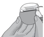
CAUTION: Ensure that the lead is fully inserted before tightening the set screw to prevent lead damage
