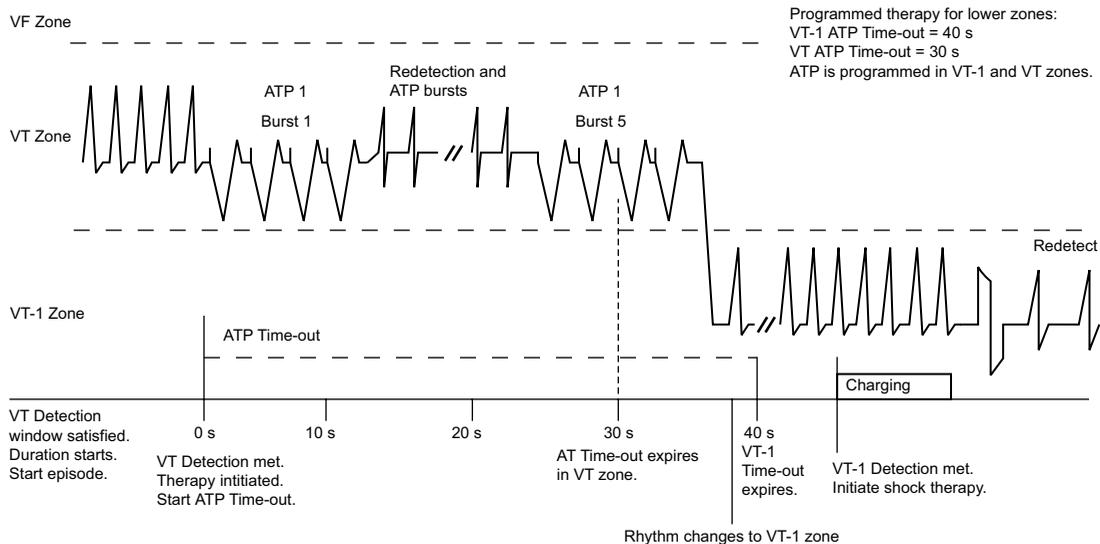
**Figure 4-20. ATP Time-outs, 3-zone configuration**
