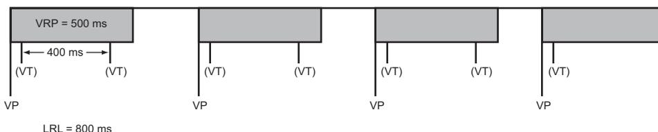
**Figure 5-29. Ventricular undersensing due to VRP**
