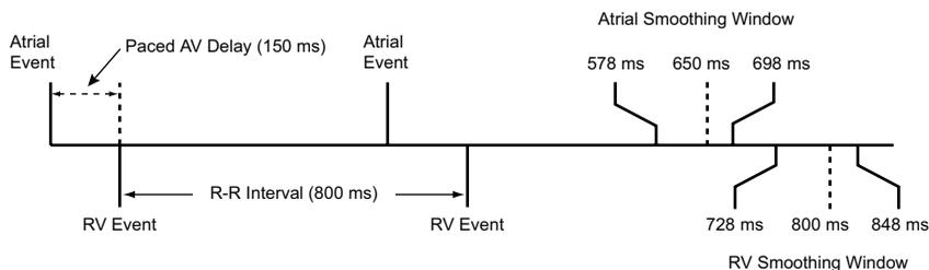
**Figure 5-15. Rate smoothing synchronization window**
