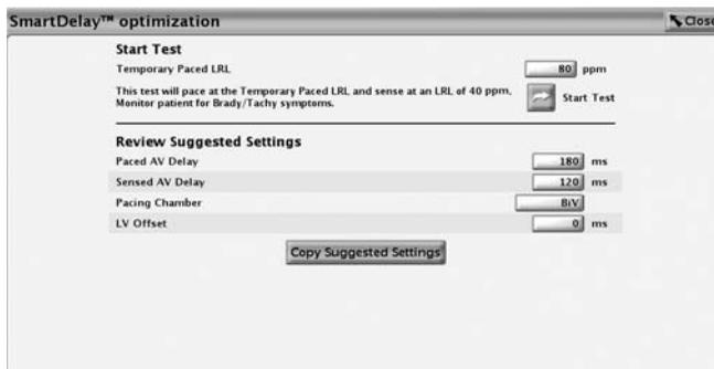
**Figure 5-20. SmartDelay optimization screen**
