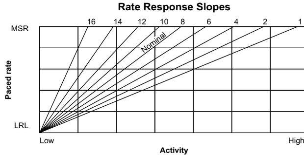
**Figure 5-9. Response Factor and paced rate**
