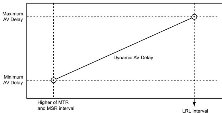
**Figure 5-17. Dynamic AV Delay linear relationship**
