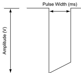
**Figure 5-3. Pulse waveform**
