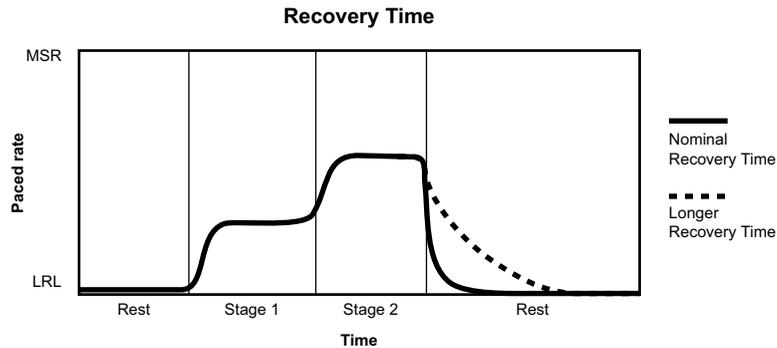
The figure shows the effect of higher and lower settings during a theoretical two-stage exercise test.
