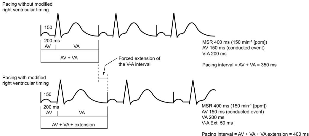
The pulse generator's timing algorithm provides effective pacing at the MSR with intrinsic ventricular conduction. Extending the VA interval prevents the A pace from exceeding the MSR at high rates.
