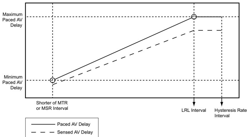
**Figure 5-19. Dynamic and Sensed AV Delay as a function of the escape interval**
