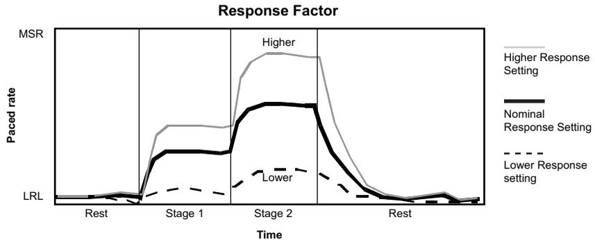
This figure shows the effect of higher and lower settings during a theoretical two-stage exercise test.
