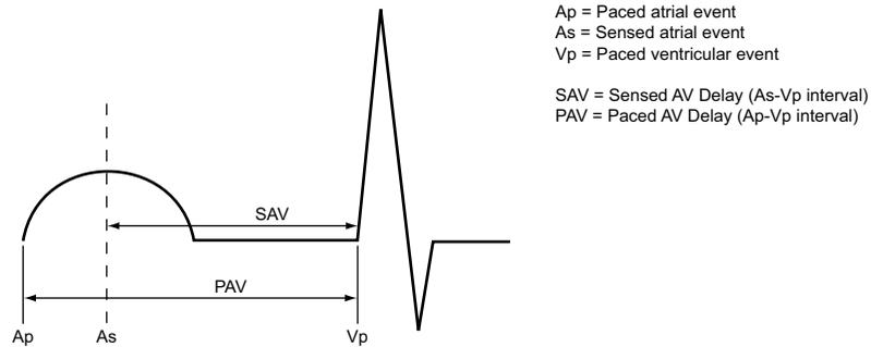
**Figure 5-18. Sensed AV Delay**
