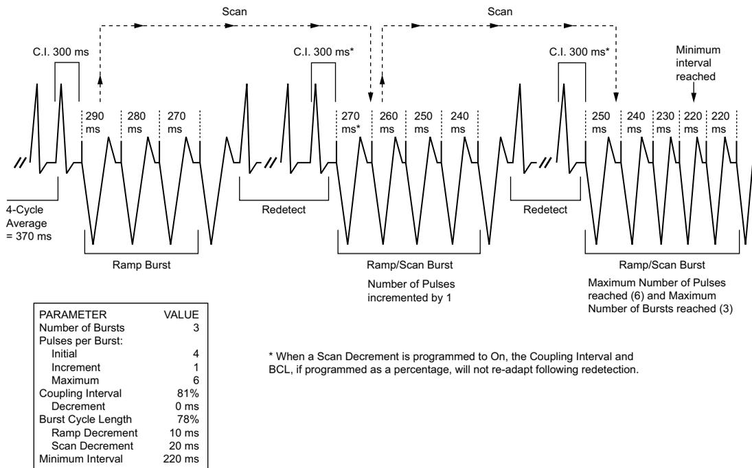
**Figure 4-18. Ramp/Scan scheme, interaction of ATP parameters**
