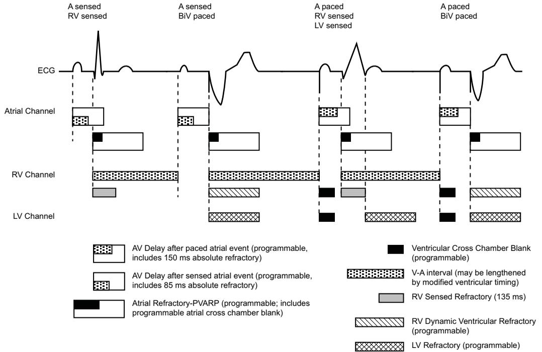
**Figure 5-24. Refractory periods, dual-chamber pacing modes; BiV**
