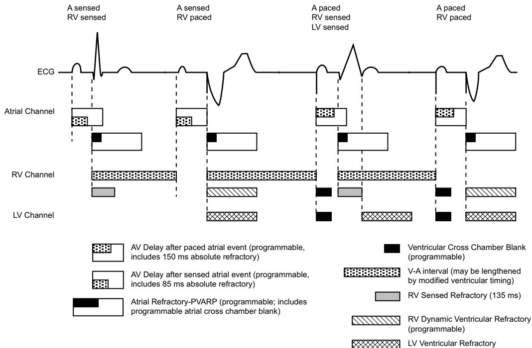
Figure 5-23. Refractory periods, dual-chamber pacing modes; RV only
