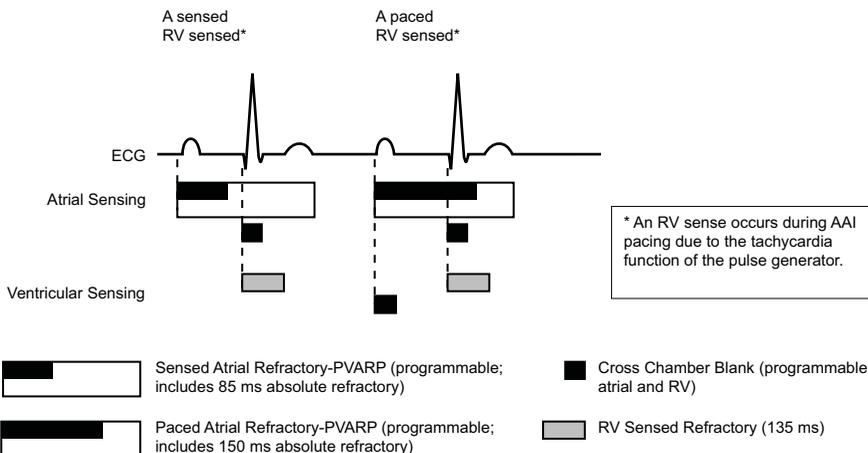
Figure 5-26. Refractory periods, AAI pacing mode
