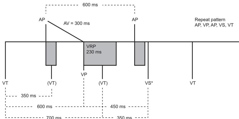
Figure 5-30. Ventricular undersensing due to V-Blank after A-Pace
