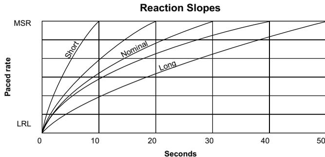
**Figure 5-7. Reaction Time and paced rate**
