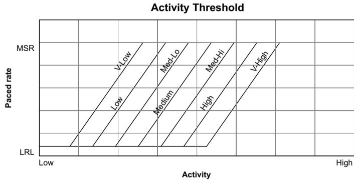
**Figure 5-5. Activity Threshold and rate response**
