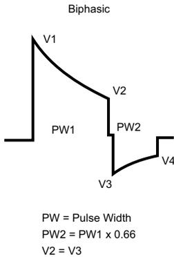
**Figure 4-21. Biphasic waveform**
