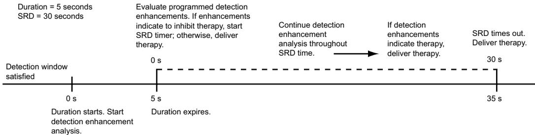
**Figure 3-21. Combination of Onset OR Stability, SRD programmed on**
