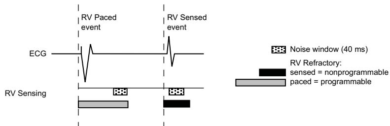
**Figure 5-27. Refractory periods and noise windows, RV**
