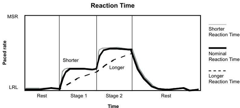
**Figure 5-8. Reaction Time in exercise test**
