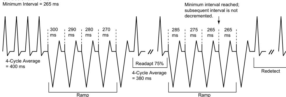
**Figure 4-16. Adaptive Ramp Scheme, Coupling Interval Decrement and Scan Decrement programmed to 0**
