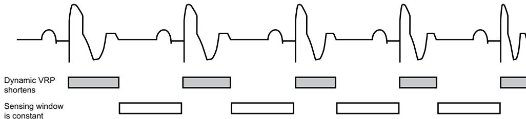
**Figure 5-22. Relationship between ventricular rate and refractory interval**
