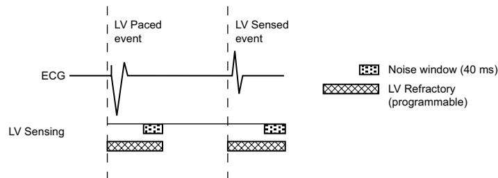
**Figure 5-28. Refractory periods and noise windows, LV**
