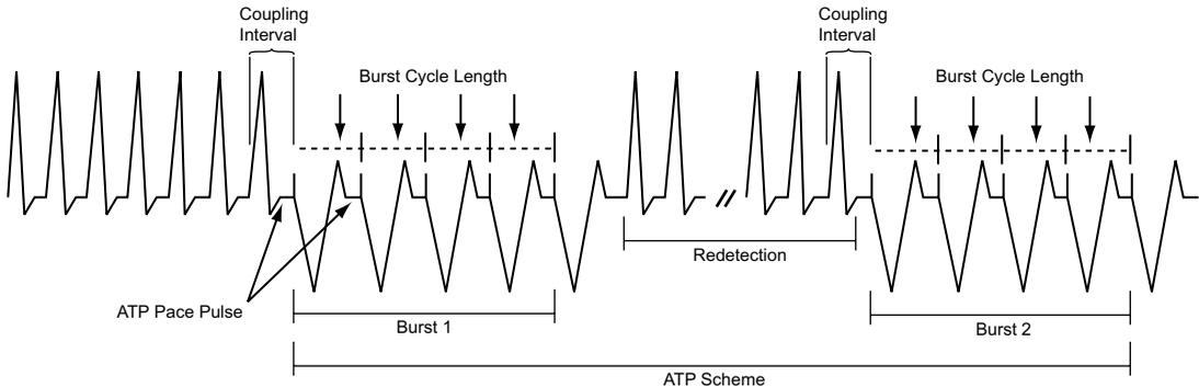
**Figure 4-11. ATP therapy basic parameters are Coupling Interval, Burst Cycle Length, Number of Bursts, and Number of Pulses within each burst.**
