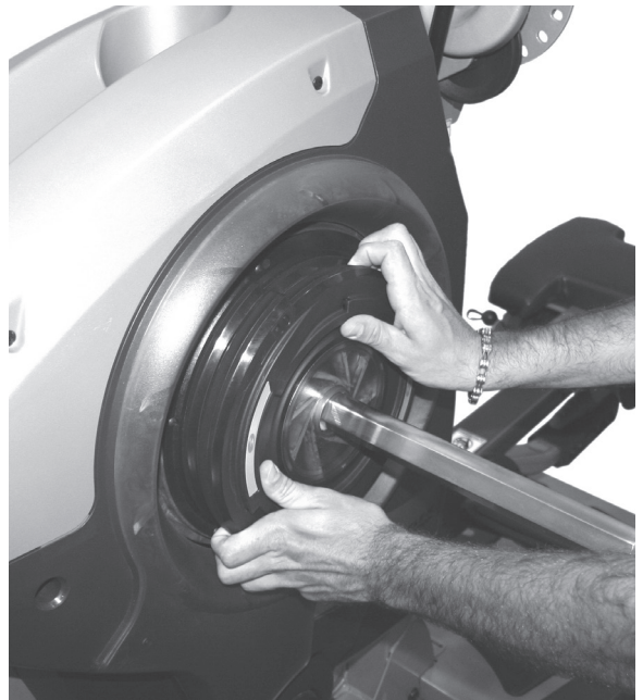
Step 2: While pressing pack towards machine, turn counterclockwise about 10 degrees until all six plate tabs lock into place. Then turn clockwise until index marks are aligned.
