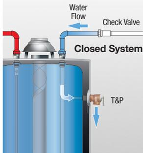
In a closed system, and without taking the proper precautions, the expanded water has no place to go. The resulting pressure increase will cause your water heater’s temperature and pressure (T&P) relief valve to trigger, expelling the additional pressure and water volume through the valve.
