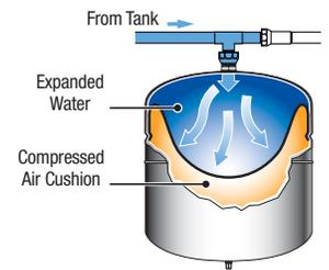
As the pressure within the water heater normalizes (typically after there’s a call for hot water within the home), the water within the expansion tank is forced back into the water heater by the diaphragm, and the potentially harmful effects of thermal expansion are eliminated.
