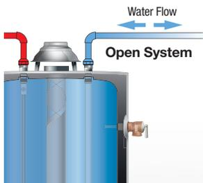
But today’s plumbing regulations require the integration of backflow preventers or check valves, primarily to keep the water in your home from the possibility of contaminating the water supply. As a result, present-day hot water systems are considered “closed” systems.
