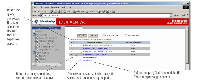
After completion of a query, here is how a typical Browse Chassis page looks with the module hyperlinks active and the Display compact check box unchecked.
