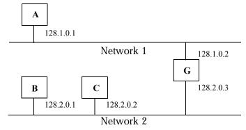
When host B with IP address 128.2.0.1 communicates with host C, it knows from C's IP address that C is on the same network. In an Ethernet environment, B can then resolve C's IP address into a hardware address (MAC address) and communicate with C directly.
