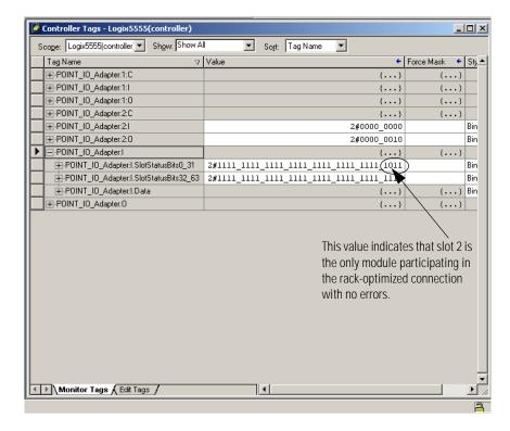
Use the controller tags in your ladder program to read input data or write output data.
