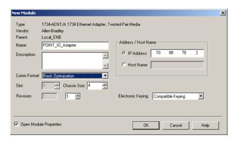
**4.** Enter values for Name, IP Address, Comm Format, Chassis Size, Electronic Keying, and Revision, noting we used the following values.
