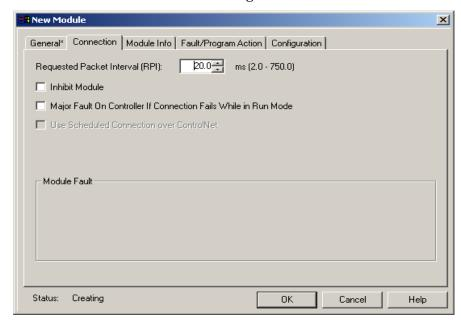
**8.** From the New Module dialog, enter 50 for the requested packet interval (RPI).
