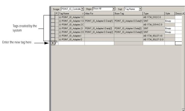
The Controller Tags dialog opens. You see the tags created for the 1734-AENT adapter and digital I/O modules.
