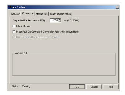
**6.** Verify that the requested packet interval (RPI) is appropriate for your system (10 ms for this example). You use this value for the rack-optimized connection to the I/O modules.
