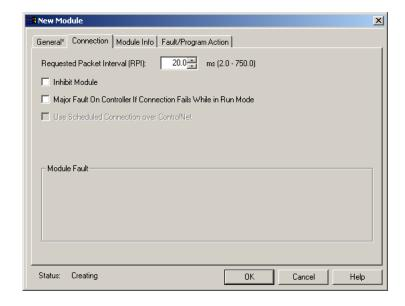
**6.** Enter 50 for requested packet interval (RPI) to set how often you exchange data with the 1734-AENT adapter.
