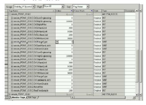
**5.** Click the value 2 and change it to 0, which changes the voltage range to -10 to +10V dc for channel 0.
