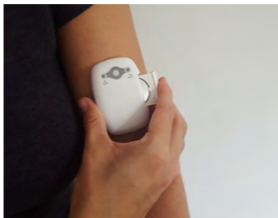
2k Slide fully charged EZ battery tray into monitor
