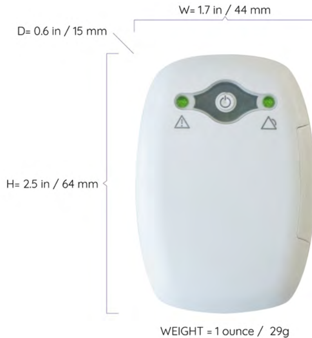
5a Technology: surface electromyography (sEMG)
