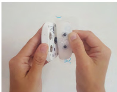
2h Snap a new Electrode Patch into monitor
