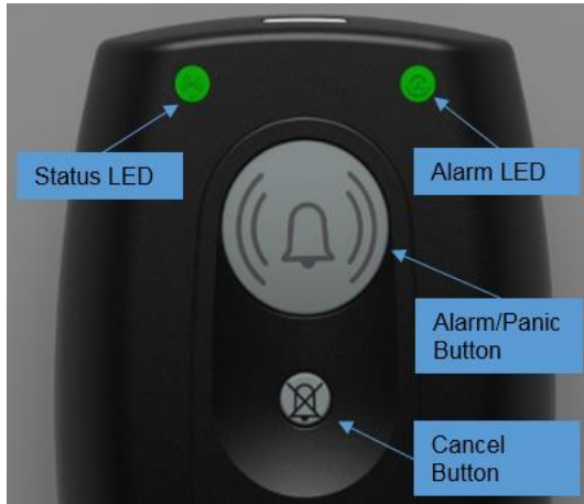
Figure 3H. The SPEAC® Detection Device Front View
