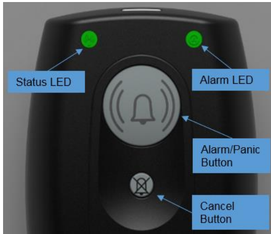
Figure 3F. The SPEAC® Detection Device Front View
