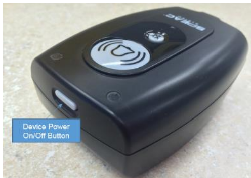
Figure 4H. SPEAC ® Detection Device ON/OFF Button
