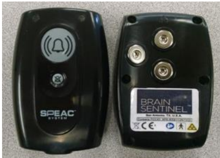
Figure 4P. SPEAC® Detection Device Enclosure
