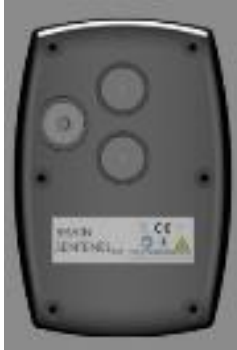
Figure 4O. SPEAC® Detection Device Electrode Sockets
