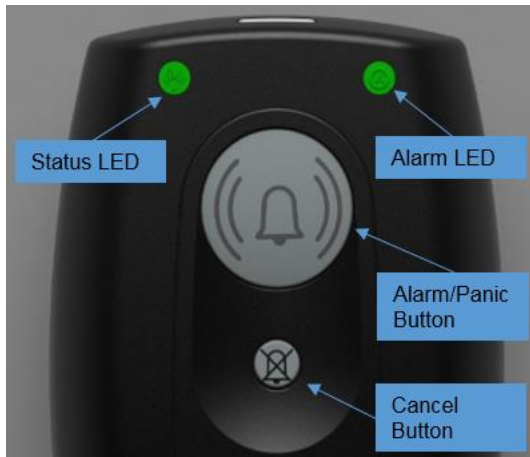
Figure 3C. The SPEAC® Detection Device Front View
