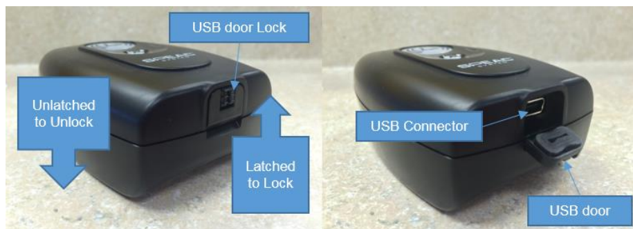
Figure 4N. Detection Device USB Door and USB connector
