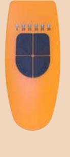
buttons to select the required run time. To deactivate and lock the remote.
