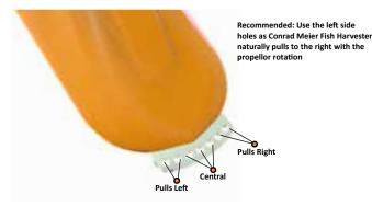
**Tip:** Clip the carabiner to the left side hole to compensate for the natural pull to the right created by the rotating propellor.
