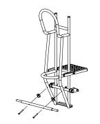
Secure axle in place using 2 x M8 screws, 2 x axle location clips & 2 x M8 nuts
