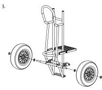
To fit wheels, slide 1 x washer, 1 x wheel & remaining washer onto axle. Repeat for opposite side
