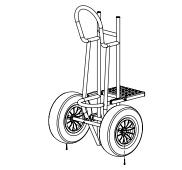
Lock in place using a split pin on each end of the axle
