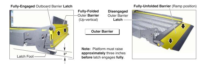
The latch disengages the barrier when the platform lowers fully (reaches ground level) and the latch foot contacts the ground (latch raises above the barrier).
