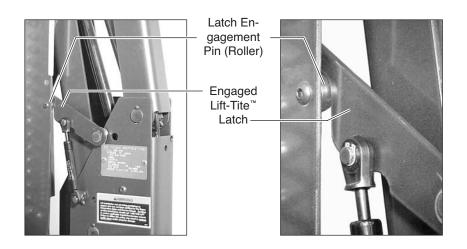
vent the platform from unfolding from the stowed position in the event of platform drift. Due to the "all-hydraulic" operation of the dual-cylinder NL, hydraulic fluid expansion, contraction or seepage may occur. Any of these conditions may result in platform drift (failure to hold the platform in the folded or raised position). Platform drift may occur during lift shipment and/or between extended periods of non-lift use.
