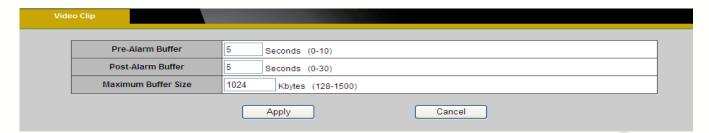
This function is used to determine when video clips will be recorded and stored after an event is triggered.
