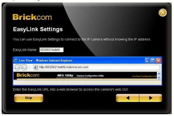
EasyLink™ is a unique Brickcom function which allows users to assign a unique EasyLink name to their network camera's IP address. There is no need to configure the router to open up ports or remember hard-to-memorize IP addresses. Users can log onto [uniqueEasyLinkname].mybrickcom.com to view the camera's web GUI and live view.
