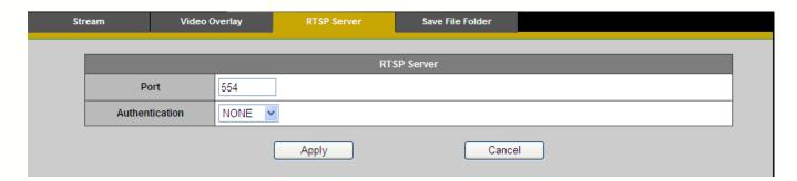
To utilize RTSP authentication, the user must first set a password for the camera. RTSP (Real-Time Streaming Protocol) controls the delivery of streaming media. By default the port number is set to 554.
