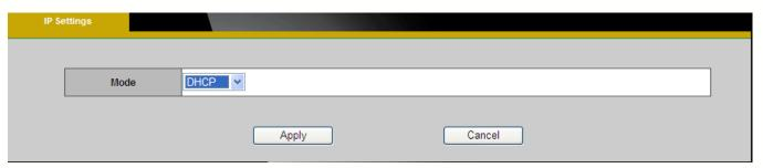
1. **DHCP** –If this option is selected, the camera will automatically obtain an available dynamic IP address from the DHCP server each time it connects to the LAN.
