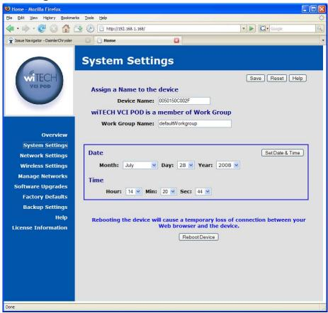
You can assign a name to the device that will be shown on the device discovery utility screen in place of the default serial number. You may also wish to set the date and time on the device.
