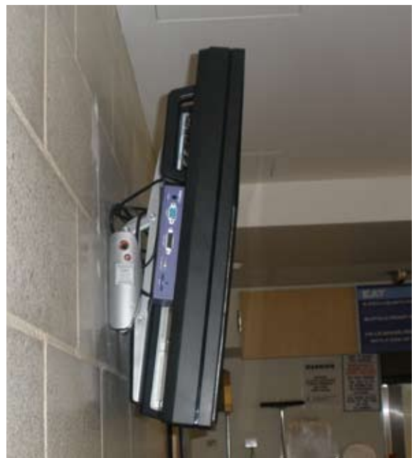
BrightSign’s slim player easily fits behind video screens, out of sight of customers.
