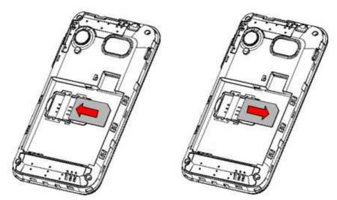
**Warning:** Damages could happen to your SIM card if the device is not switched off when taking out of the SIM card.
