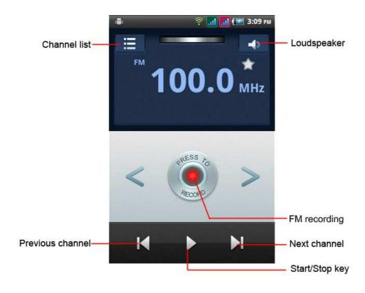
**Attention:** this handset doesn't have a built-in antenna. If you want to listen to the radio, please insert the headphone first. Pressing the side key can adjust the volume.
