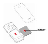
Note: Do install the battery as per the diagram so as prevent the battery contact patch being damaged. (See figure below)
