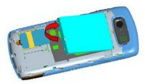
When installing the battery, insert the metal teeth at the top of the battery into corresponding slot of the mobile phone, and then press the battery down to install the battery in place. The battery must be ensured to be installed before power on. ■ Finally install the rear cover of the mobile phone.
