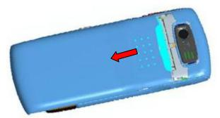
Dig out the bottom of the battery and get the battery out.
