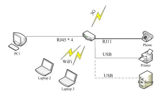
When 3G Only Internet connection is applied, the device is connected to the Internet through the built-in 3G Modem, All of the four RJ45 connectors will be used to build wired LAN network. At the same time, network sharing function can be achieved through WLAN for any terminal devices that support WiFi. Voice service is provided via CS domain by connect fix-line phone to
