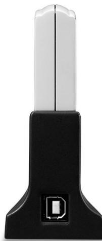
And your Adapter comes with a USB cable that has two different types of connectors – type A & type B. Type A connector of the USB cable plugs into your notebook/desktop PC's USB port. And type B connector of the USB cable connects to the USB port of your USB Wireless Network Adapter.
