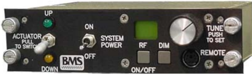
Figure 10: Control panel with actuator switch
