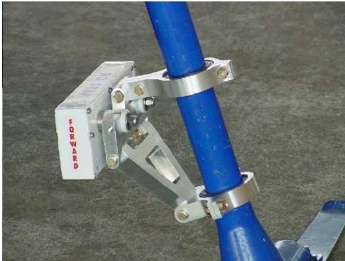
Figure 1. Cross-tube strut mount
