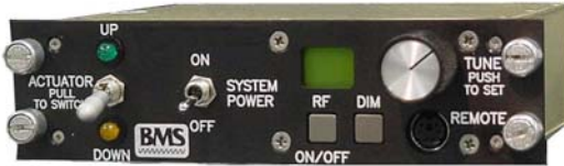
Figure 10: Control panel with actuator switch
