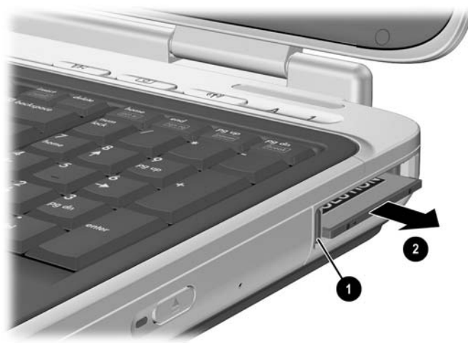
Removing a PC Card
