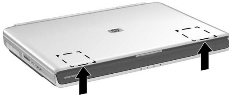
Wireless antennae location
