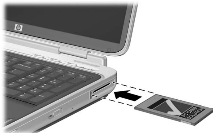
Inserting a PC Card
