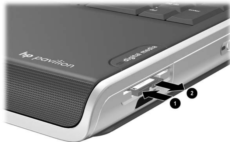
Releasing and removing a digital media card
