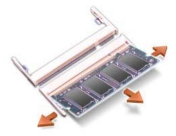
**NOTICE:** If you need to install memory modules in two connectors, install a memory module in the connector labeled "SLOT 1" before you install a module in the other connector.
