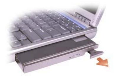
**3** Insert the new device into the bay, push the device until you feel a click, and push the device latch release in so that it is flush with the computer.
