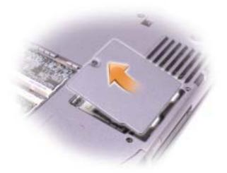
7 Place your finger under the cover at the indentation, and lift and slide the cover open.
