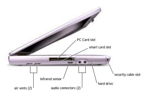
AIR VENTS — The computer uses an internal fan to create airflow through the vents, which prevents the computer from overheating.
