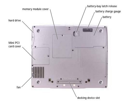
MEMORY MODULE COVER — Covers the compartment that contains the memory module(s). See "Adding Memory" on page 108.
