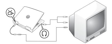
To connect the computer to a television that has a composite video input only, Dell provides a composite TV-out adapter cable. Before you begin, ensure that you have the following cables:
