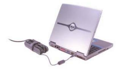
The AC adapter converts AC power to the DC power required by the computer. You can connect the AC adapter with your computer turned either on or off.
