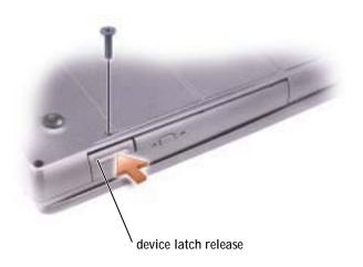
4 Use a #1 Phillips screwdriver to remove the device screw from the bottom of the computer.
