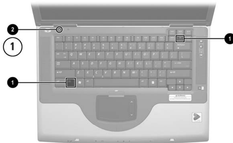
Identifying the Fn and num lk keys and the num lock light
