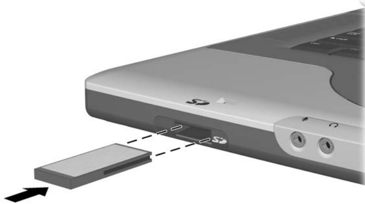
Inserting an SD Card or MMC
