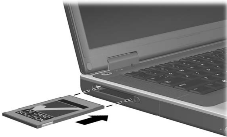
Inserting a PC Card
