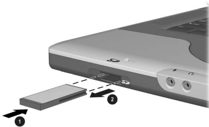
Releasing and removing an SD Card or MMC
