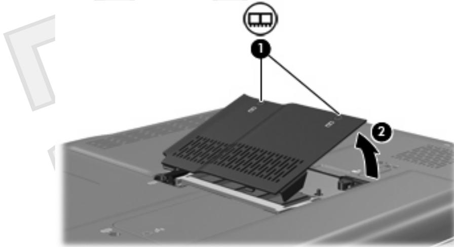
9. If you are replacing a memory module, remove the existing memory module:
