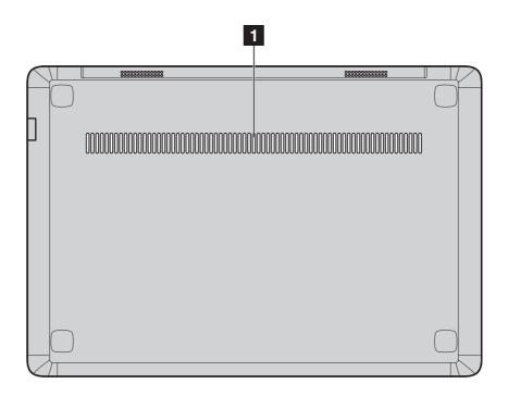
**Air inlet louvers** Make outside air go inside the computer through the louvers.
