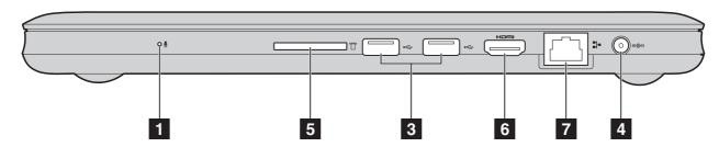
**Built-in** The built-in microphone (with noise reduction) can be used for video conferencing, voice narration, or simple
