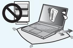
**Do not use the computer in a badly ventilated location such as on bedding, on a pillow or cushion, etc, and do not use it in a location such as room with floor heating as it may cause the computer to overheat.**
