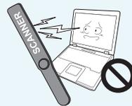
**Avoid exposing a drive to magnetic fields. Security devices with magnetic fields include airport walk-through devices and security wands. The airport security devices that check carry-on luggage, such as conveyor belts, use x-rays instead of magnetism and will not damage a drive.**
