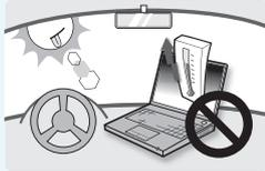
**Never heat the product(or battery) or put the product(or battery) into a fire. Do not put or use the product(or battery) in a hot location such as a sauna, inside a vehicle exposed to the heat, and so on.**
