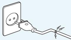
**Do not use a damaged or loose main plug or power cord or power outlet.**
