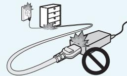
**Do not place heavy objects or step onto the power cord or AC adapter to avoid damaging the power cord or AC adapter.**
