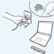
**Disconnect all cables connected to the computer before cleaning it. If your notebook is external & removable battery type, remove the external battery.**
