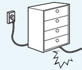
**Do not bend the power cord excessively or do not place a heavy object over the power cord. It is especially important to keep the power cord out of reach of infants and pets.**
