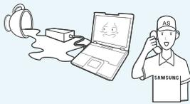
**If water or another substance enters the power input jack, AC adapter or the computer, disconnect the power cord and contact the service center.**
