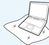
**Avoid blocking the vent at the bottom or side of the computer when using it on a bed or cushion.**
