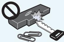
**Take care not to allow metal objects such as a key or clip to touch the battery terminal (metal parts).**
