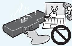
**If liquid leaks out of the product(or battery) or there is a funny smell coming from the product(or battery), remove the the product(or battery) the computer and contact a service center.**
