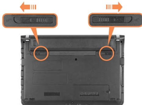
**3** To install the battery again, slide the battery into the system. The battery latches move inwards and fix the battery automatically.
