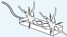
**Do not exceed the standard capacity (voltage/current) of a multiplug or power outlet extension when using it for the product.**
