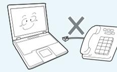
**Do not connect a phone line connected to a digital phone to the modem.**
