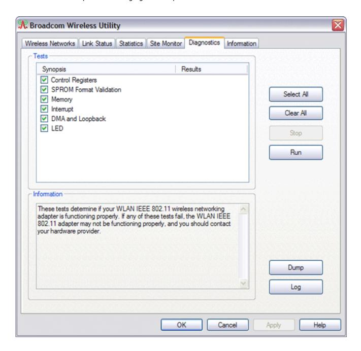
If your Broadcom 802.11 Network Adapter fails any of the diagnostics tests, go to <a href="http://www.broadcom.com/">http://www.broadcom.com/</a> for technical support.
