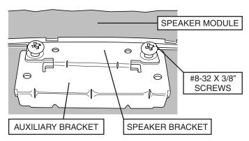
4. Attach AUXILIARY BRACKET (loose bracket in parts bag) to SPEAKER BRACKET (attached to SPEAKER MODULE). Partially install (2) #8-32 X 3/8" SCREWS (short screws from parts bag) through larger holes in speaker bracket and into auxiliary bracket - only so ends of screws are flush with bottom surface of auxiliary bracket. Note: Installing screws below flush will make the next steps more difficult.
