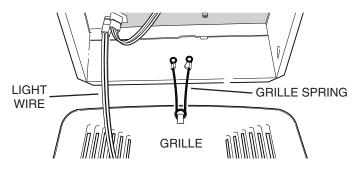
Remove fan GRILLE by squeezing two GRILLE SPRINGS and sliding them out of their mounting slots on each side of the fan housing. Disconnect LIGHT WIRE from fan (if fan is equipped with a light). Set grille assembly aside for now.
