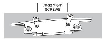
4. Partially install (2) #8-32 x 5/8 screws (included) into threaded holes in speaker bracket - only so ends of screws are flush with bottom surface of speaker bracket. Note: Installing screws below flush will make the next couple of steps difficult.
