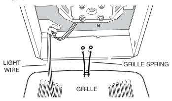
2. Remove fan **GRILLE** by squeezing two **GRILLE SPRINGS** and sliding them out of their mounting slots on each side of the fan housing. Disconnect **LIGHT WIRE** from fan (if fan is equipped with a light). Set grille assembly aside for now.
