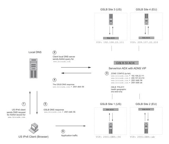
The GSLB controller makes decisions based on the GSLB policy. In the example above, both the IPv6 VIPs were healthy, so client was directed to the IPv6 VIP that was geographically closer based on the configured policy. If the VIP at the geographically closer site (the US site) was down, the GSLB controller would direct traffic to the EU site.
