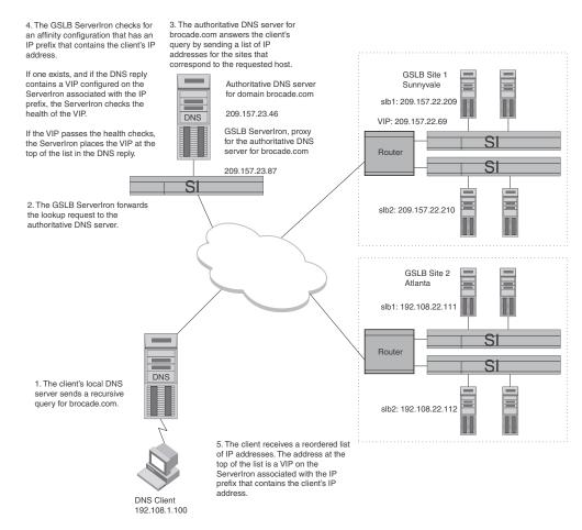
In Figure 5, the client's IP address is within the configured attinity prefix, so the ServerIron ADX checks the DNS reply for a VIP configured on the ServerIron ADX associated with the prefix:
