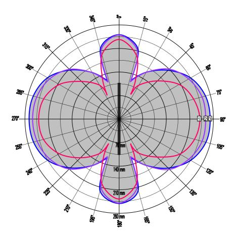
Case 2: The following diagram shows the reading range of the transponder card in the upper reference plane. This is the recommended position for an optimal reading range for this transponder card orientation.
