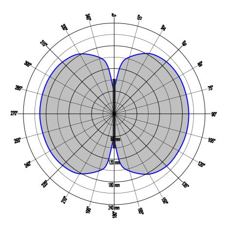
Case 2: The diagram below shows the reading range depending on the transponder position.
