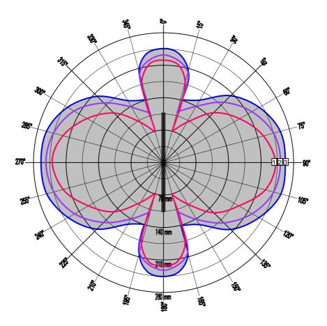
Case 2: The following diagram shows the writing range of the transponder card in the upper reference plane. This is the recommended position for an optimal writing range for this transponder card orientation.
