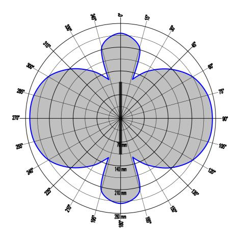
Case 1: The diagram below shows the reading range depending on the transponder position.
