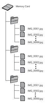
If the memory card is used with the scanner for the first time, the scanner creates a folder named "FotoIMG" in the root directory to store the scanned image files. Each image file has a prefix "IMG\_" followed by a 4-digit serial number in the sequence the image is stored.
