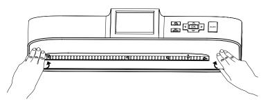
Insert the white side of the cleaning stick all the way into the paper slot on the back of the scanner. Slide it back and forth several times to clean any debris out of the area.
