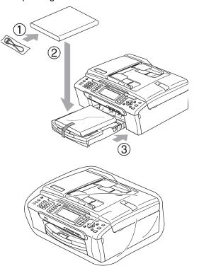
Pack the printed materials in the original carton as shown in the illustration. Do not pack the used ink cartridges in the carton.
