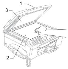
2 In the ADF unit, clean the white bar (1) and the glass strip (2) with a lint-free cloth moistened with a non-flammable glass cleaner.
