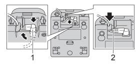
Plug the adapter into the AC power outlet.
