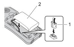
4 Place the battery in the correct position.
