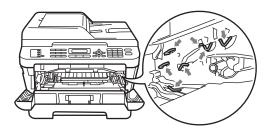
3 Push down the green lock lever and take the toner cartridge out of the drum unit. Clear the jammed paper if there is any inside the drum unit.
