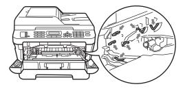
Clean the corona wire inside the drum unit by gently sliding the green tab from right to left and left to right several times.
