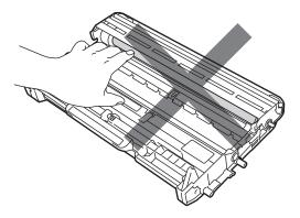
Wait to unpack the new drum unit until immediately before you put it in the machine. Exposure to direct sunlight or room light may damage the drum unit. 6 Put the toner cartridge firmly into the new drum unit until you hear it lock into place. If you put the cartridge in properly, the green lock lever will lift automatically.
