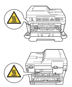
2 Slowly take out the drum unit and toner cartridge assembly. The jammed paper may be pulled out with the drum unit and toner cartridge assembly, or this may release the paper so you can pull it out inside of the machine.
