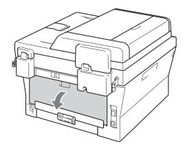
4 Pull down the tabs at the left and right hand sides to open the fuser cover (1).
