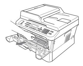
4 Push down the green lock lever and take the toner cartridge out of the drum unit.
