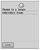
This message is displayed when the machine is in embroidery mode and the small frame is attached, and the selected pattern does not fit in the small
