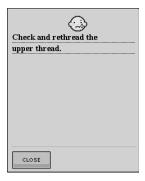
This message is displayed when the upper thread is broken or not threaded correctly, and the "Start/Stop" button or the "Reverse/ Reinforcement Stitch" button is pressed.
