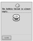
This message is displayed when the bobbin thread is running out.
