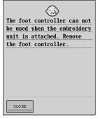
This message is displayed when the foot controller is pressed while the embroidery unit is attached.
