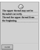
This message is displayed when it seems that the upper thread has not been threaded correctly.
