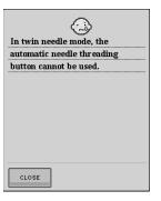
This message is displayed when the automatic needle threading button is pushed while twin needle sewing is set.
