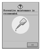
Once this message appears, it is recommended to take your machine to an authorized retailer for a regular maintenance check. Although this message will disappear and the machine will continue to
