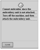
This message is displayed when the "Start/Stop" button is pushed and the machine is in embroidery mode, but the embroidery unit is not attached.
