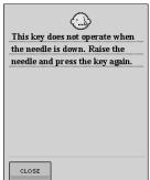
This message is displayed when a key on the LCD display is touched while the needle is in the down position.
