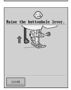
This message is displayed when the buttonhole lever is down, a stitch other than a buttonhole is selected, and the "Start/ Stop" button or the "Reverse/ Reinforcement Stitch" button is pushed.
