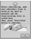
This confirmation message appears after the machine is turned on and the carriage of the embroidery unit has moved to its initial position.
