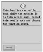
This message is displayed when the machine is in twin needle mode and a pattern that cannot be sewn with the twin needle is selected.
