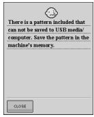
This message is displayed when you try to save a copyright protected pattern to USB media/ Computer. According to copyright laws, patterns that are illegal to reproduce or edit cannot be saved to floppy disks. If this message displays, save the pattern in the machine's memory.
