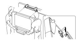
Attach the tray by sliding its slots over the two brackets on the front of the copyboard above the printer.
