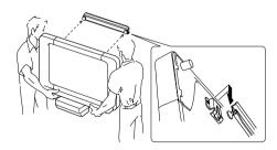
With the copyboard mounted on the wall, remove the two screws on the bottom of the unit with a screwdriver. Attach the long ends of the two enclosed L-shaped brackets to the bottom of the unit using the two screws.
