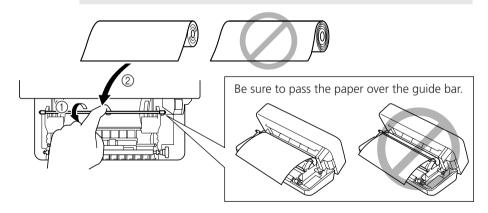
Release the bar while making sure that the paper feeds over it, and then lift the paper compartment cover with both hands and firmly close it.
