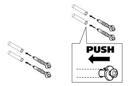
Tighten <u>each screw</u> (by turning it clockwise) approximately 20 turns.
