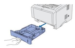
2 While pressing the paper guide release lever, slide the adjusters to fit the paper size. Check that the guides are firmly in the slots.
