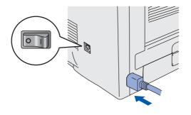
Plug the AC power cord into an AC outlet. Turn the power switch on.
