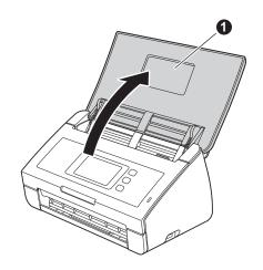
Pull the Output Tray out of the machine **1** and then unfold the Document Stopper **2**.
